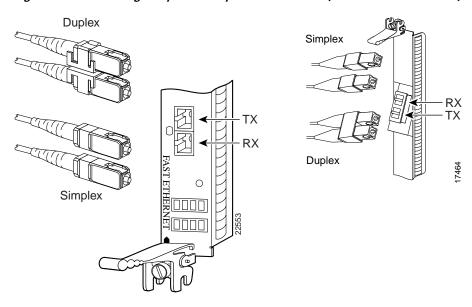
Figure 42 Attaching Simplex or Duplex Fiber Cables (Line Card Port or GBIC)
